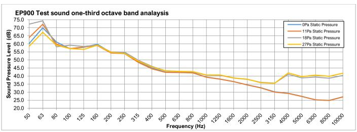
Testing was conducted by AMCA International. Product tested to AMCA Standard 300, Figure 2 Setup, Installation Type A, equivalent to ISO 13347.
