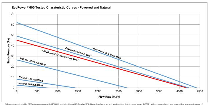
wind across the specimen. Wind assisted tests performed by Edmonds on Edmonds in house test equipment. Wind assisted performance testing is outside the scope of AMCA's test standards.
