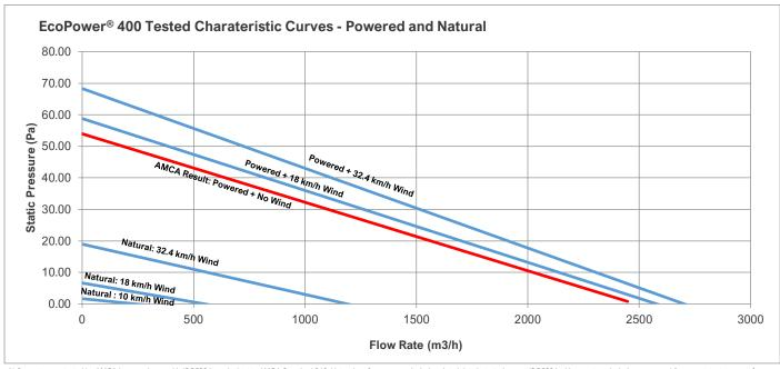
Airflow rates are tested by AMCA in accordance with ISO5801, equivalent to AMCA Standard 210. Natural performance and wind assisted data is tested as per ISO5801 with an external wind source providing a constant source of wind across the specimen. Wind assisted tests performed by Edmonds on Edmonds in house test equipment. Wind assisted performance testing is outside the scope of AMCA's test standards.
