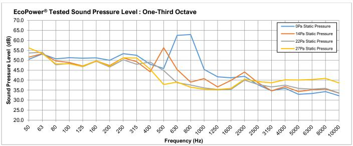
Testing was conducted by AMCA International. Product tested to AMCA Standard 300, Figure 2 Setup, Installation Type A, equivalent to ISO 13347.
